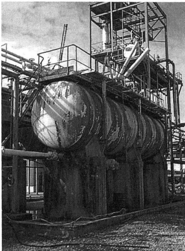
Figure 2. Shows monomer feed tank and vacuum system to reactors.
